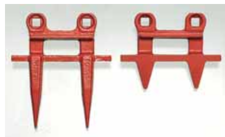
Choose standard or stub guards to suit your local crop conditions. Standard guards are streamlined for better penetration in fine grasses and thick undergrowth. Stub guards are recommended for use when cutting dead or wet undergrowth since they will not plug as readily.
