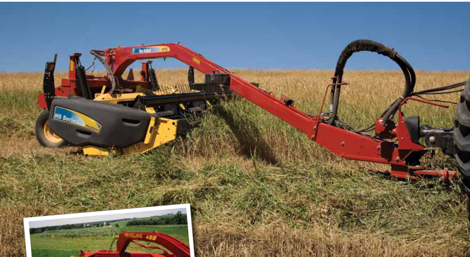
In 1983, New Holland introduced the 499. This Haybine model featured pivot-tongue convenience and the unique Rolareel header swept crop from a wide, 12-foot cut into the conditioning rolls without the need for an auger.
