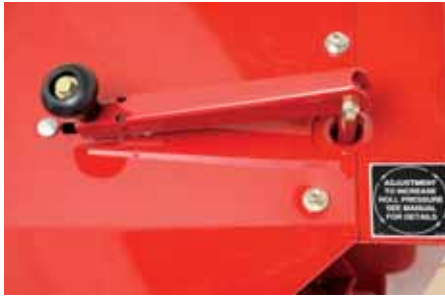
Roll pressure is adjusted quickly and easily with the turn of a crank. No tools needed! Adjustment is infinite so you can choose the exact degree of conditioning you need.
