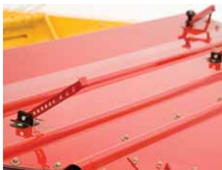
Change from swath to windrow in seconds! Just use the handy lever to adjust the swath gate and you can change from producing a narrow 36-inch windrow to a fast-drying swath up to 96 inches wide (100 inches wide on the 499, 72 inches wide on the 472) or anything in between. The H7150 also features adjustable windrow shields to custom-build windrows or swaths.
