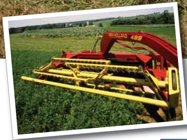
In 1983, New Holland introduced the 499. This Haybine model featured pivot-tongue convenience and the unique Rolareel header swept crop from a wide, 12-foot cut into the conditioning rolls without the need for an auger.
