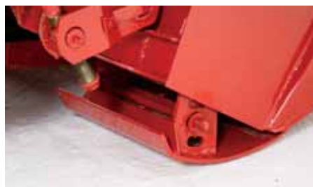
Adjustable header skid shoes allow for quick cutting height adjustment.
