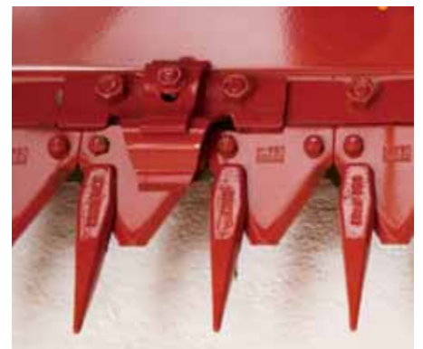
Bolt-on, over-serrated, back-hardened knife sections with adjustable hold-downs are standard equipment.
