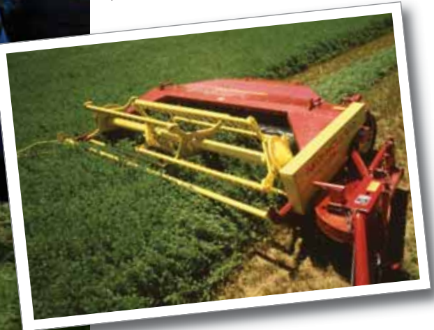
The 12-foot Haybine model 495 was introduced in 1975. It featured 110-inch-wide conditioning rolls to speed drying time, and offered a lateral transport mode.
