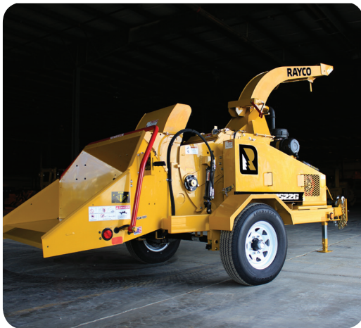
130 hp GM Gasoline Engine
