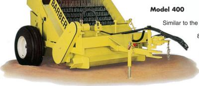
Similar to the model 400HD, the model 400 is the smallest Surf Rake<sup>®</sup>. It weighs 860 kilograms and can lift up to 1100 kilograms in its 0,75 cubic meter hopper. Its hydraulic dump discards material neatly on the ground. Within one hour, the model 400 can effectively clean up to 1,6 hectares.
