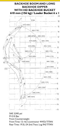
BACKHOE BOOM AND LONG TELESCOPIC DIPPER RETRACTED WITH HD BACKHOE BUCKET 610 mm (156 kg) / Loader Bucket 6 x 1
